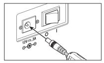
**3.** Plug the AC adapter to outlet (100 - 120 VAC  $\sim$  or 200 - 240 VAC  $\sim$  , 50 Hz/60 Hz).
